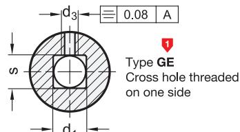
Positioning of the cross hole radially and in relation to the keyway / square for:
