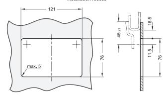
For installation, set a recess in the door, cover or hatch as shown in the outline drawing.
