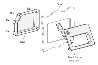
For assembly, insert the pre-assembled cam latch, on the front frame, through the front of the hole in the door, by tilting.
