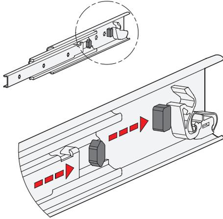
The rubber stops dampen the impact of the slide in the two end positions. This feature minimizes noise development and increases the service life. Attached to the slides in a partially concealed, partially visible manner, the stops meet each of the requirements in regards to shape, material, and hardness.
