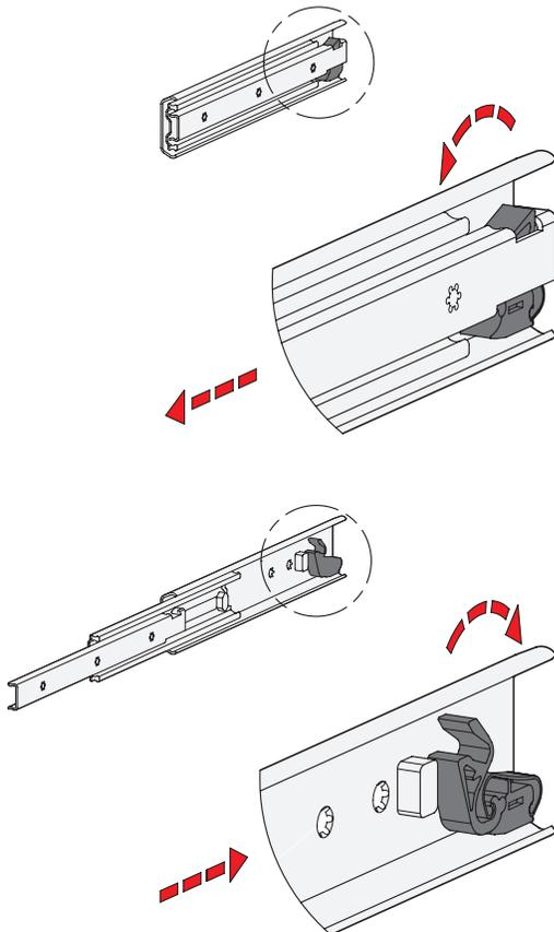
GN 1422 telescopic slides have an integrated self-retracting mechanism, which significantly improves the ease of use when closing the extensions.
