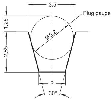
Example with three serrations and restricted indexing angle
