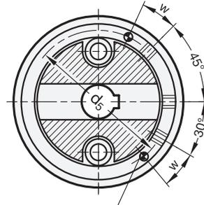
Dowel pin ISO 8750 Ø 3,5 x 7 mm protruding (only applicable when restricted indexing angle is required)
