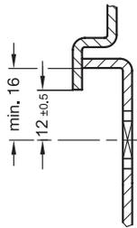
**Installation hole for punching or laser machining**
