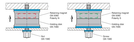
A normal holding force is achieved by combining retaining magnets with holding disks. Retaining magnets with north or south poles on the holding surface can be used equally.
