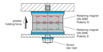
If two retaining magnets with opposite polarity are combined, an increased holding force is achieved.
