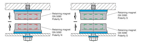
Combining two retaining magnets with the same polarity creates a repelling force.
