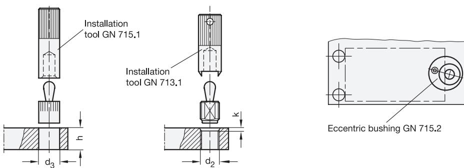
The use of a installation tool GN 715.1 or installation tool GN 713.1 is recommended for installation.
