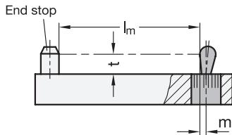
The position of the mounting hole results from the workpiece length  $l_m$  plus the hole offset  $m$ , which is calculated as shown below:
