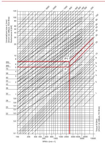
The graph shows the transferable performance N and the torques M of DIN 808 universal joints, type EW (single jointed, needle bearing) in relation to the RPM  $\rm n.$
