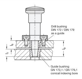
The length I<sub>7</sub> is determined by the penetration depth of the plunger pin into the cone of the bushing.
