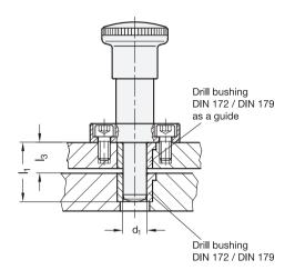
For each plunger pin diameter d<sub>1</sub> two different pin lengths l<sub>1</sub> are available.
