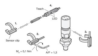
The radial position of the sensor cable can be freely determined when installing the sensor clip.
