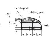
Assembly of handle part and latching part with hex head screw DIN 933-M6 or hex nut DIN 936-M6
