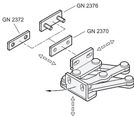
Multiple-joint hinges can be adjusted in three planes during installation. For example, this allows compensation for tolerances or establishing of required compressive forces for seals.
