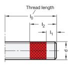
$I_1 \approx 2 \text{ to } 3 \text{ x thread pitch}$  $I_2 \approx 1.5 \text{ x d}$
